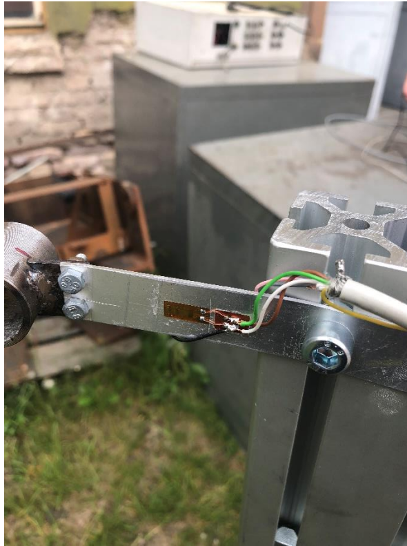
Fig. 7 Detail of applied strain gauge
