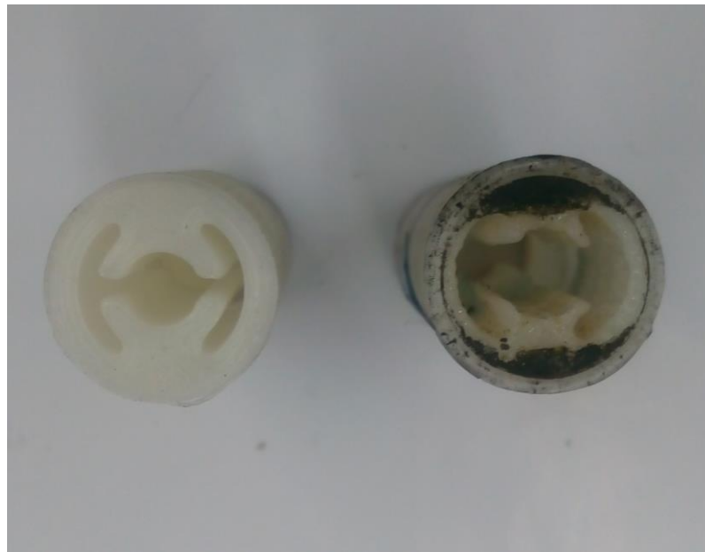
Fig. 18 left pre-combustion fuel grain, right post, PLA
