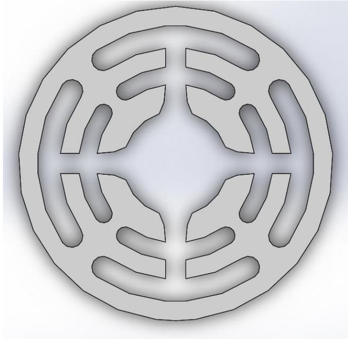
Fig. 25 Improved version of root fuel grain shape, root_2
