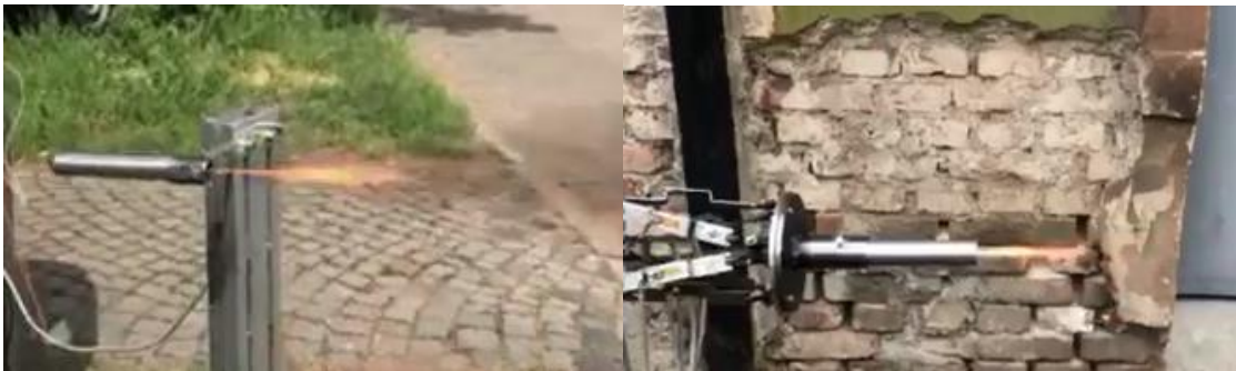
Fig. 10 Engine during run, on the left mounted in measuring apparatus, on the right in the old measuring stand
