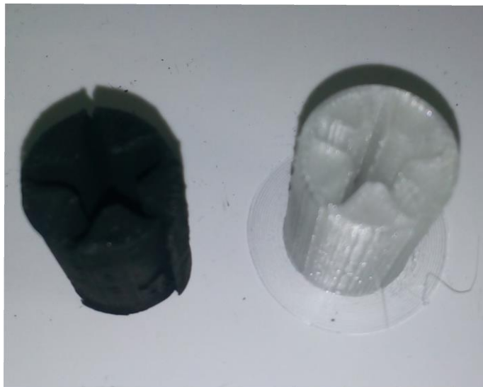
Fig. 15 Star shaped combustion port regression rate visualization
