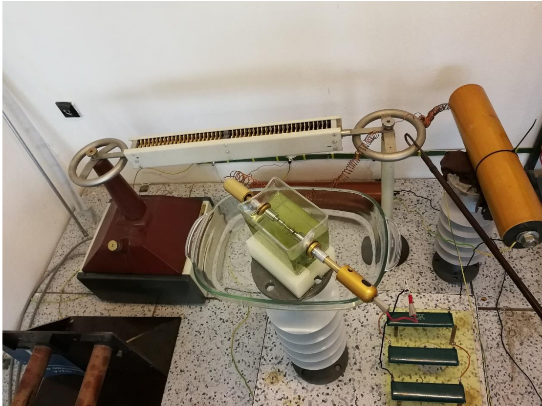
Figure 21 Testing system of XPLE for DC dielectric strength and Volt-time characteristic under DC voltage
