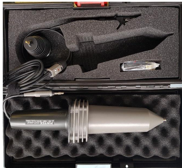
Fig. 7: High voltage probe.
