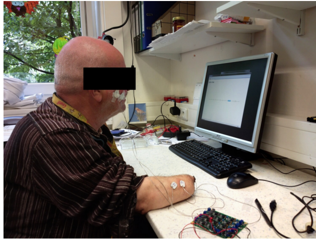
Figure 56: Disabled participant controls computer by using his EMG
