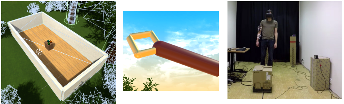
Figure 65: from the left: designed room in virtual space mapped 1:1 to real room, artificial grabber controlled by user's surface EMG signals, real room, where user can move freely and perform the task
