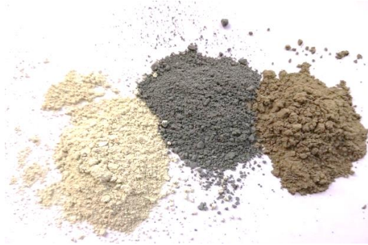
Figure 6.1.1. Raw materials used for the study. From the left: natural zeolite, silica fume, ordinary Portland cement.
