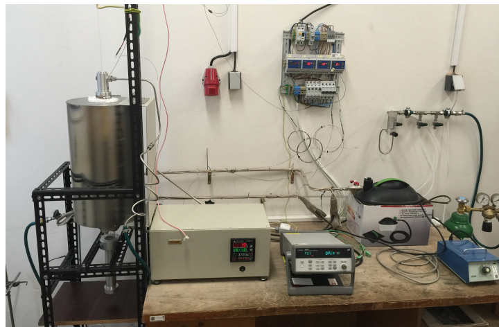
Fig. 7: Experimental setup for high temperature steam exposure in CTU laboratories
