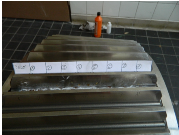
Obr. 5.11: Tenzometry na satelitu
