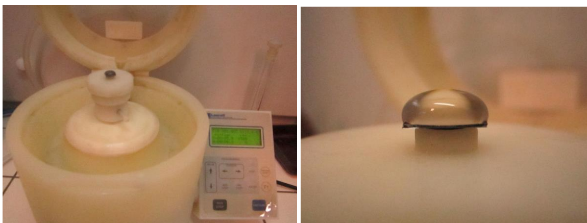
Figure 52. The spin coating mechanism to enhance nucleation density for nanocrystalline diamond growth (left) and detail of a drop of nanodiamond dispersion solution on the silicon substrate (right).
