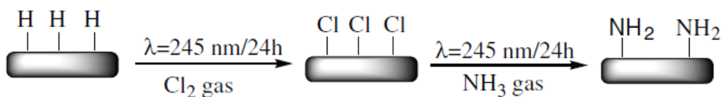
Figure 18. Preparation of an amine-terminated BDD surface in a two steps procedure, consisting on the photochemical irradiation of a hydrogenated surface with chlorine followed with ammonia gas [44].
