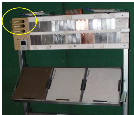
Fig. 11. Exposure and results of resistivity sensors' measurement in road tunnel.
