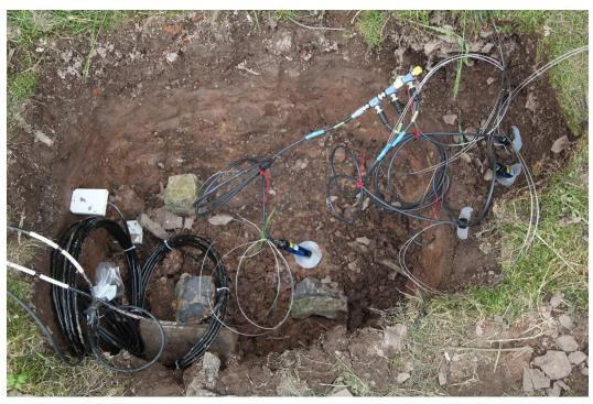
Figure 3.17 - Sensors installed in the surrounding soil at north side (Peleška, 2108)
