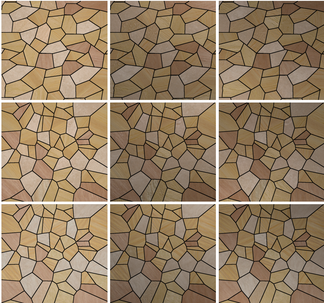
Figure 5.8: An example of a wooden floor BTF measured mosaic (top row), modeled control field mosaic with measured BTF wood (middle row), and our synthetic BTF-CMRF PV3AR model (bottom row), where the illumination azimuthal angle \phi and elevation angle \theta are successively for each column: \phi = 0^\circ, \theta = 0^\circ for the left column, \phi = 60^\circ, \theta = 60^\circ for the middle column and \phi = 60^\circ, \theta = 240^\circ for the right column.
