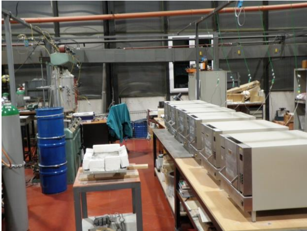
Fig. 55 Furnace used for isothermal aging
