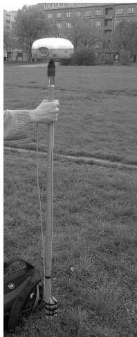
Figure 3 – a): the gradiometer probe (mounted at bottom) with (D)GPS on the top. b) gradiometer response with/without astatization
