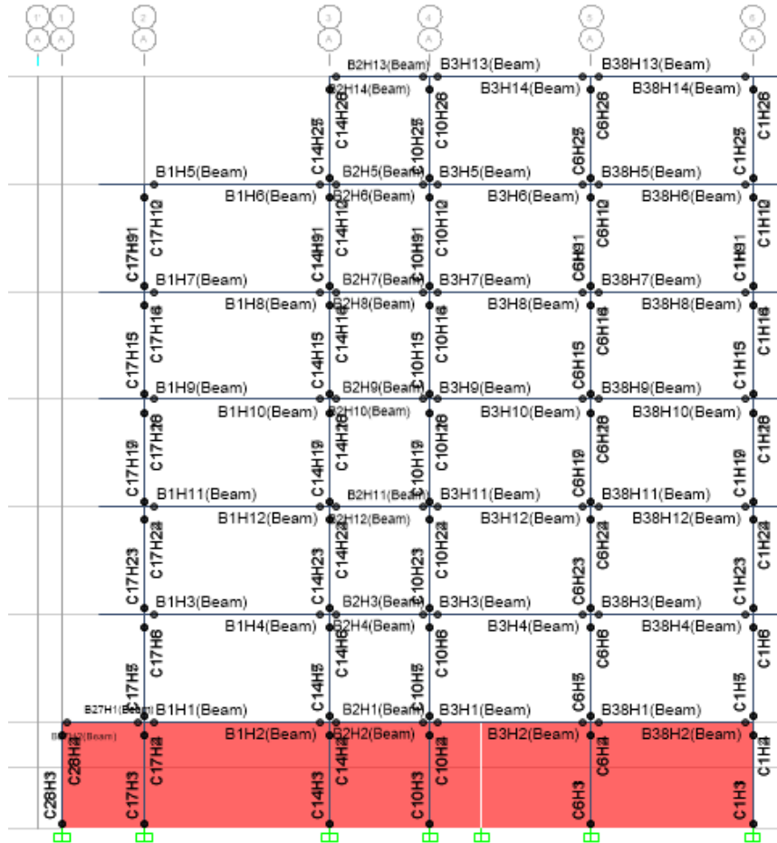
Figure 59: Nonlinear Hinge Assignments in ETABS
