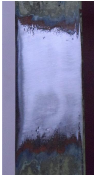
Figure 3.3 Surface for the non-destructive hardness tests
