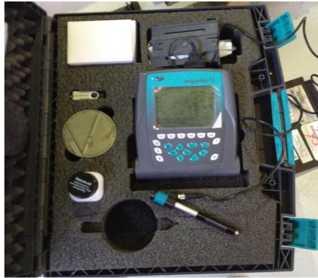
Figure 3.2 Equipment used for the non-destructive hardness tests
