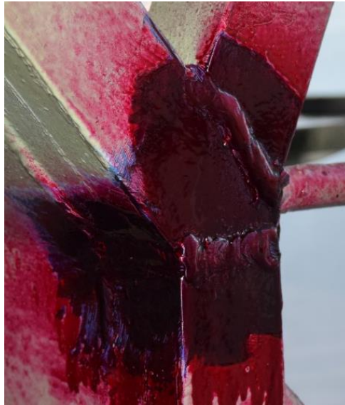
Figure 3.8 Application of the penetrant
