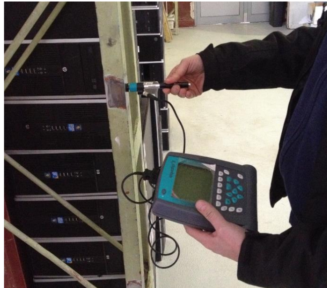
Figure 3.4 Procedure of performing the hardness test
