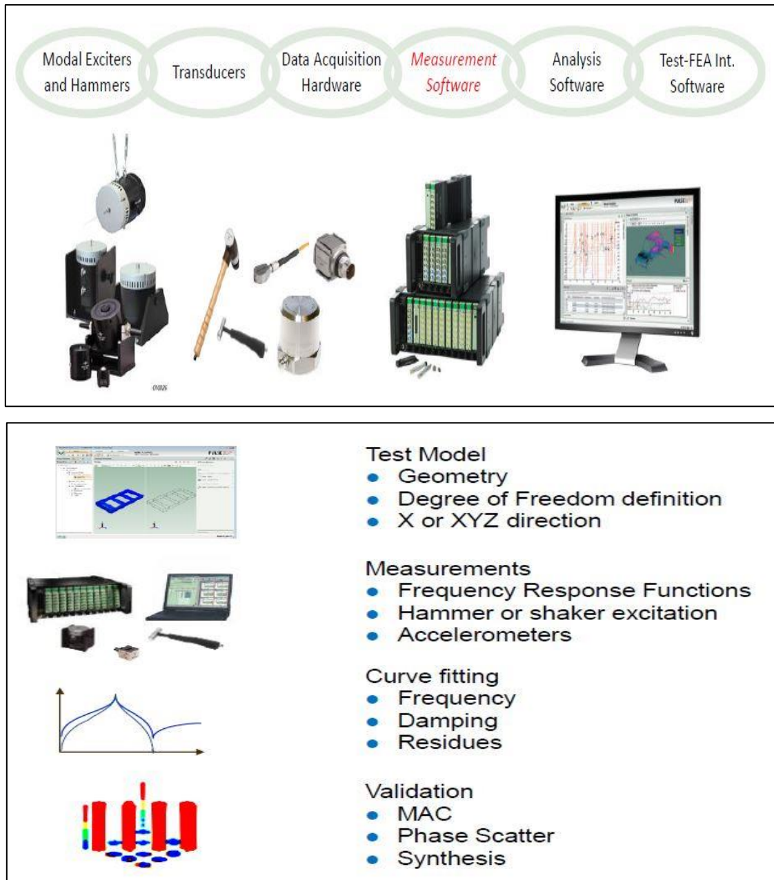
Figure A.5: The complete measurement and analysis chain [Bruel & Kjaer manual: Access code: 636 832 431; 2017].
