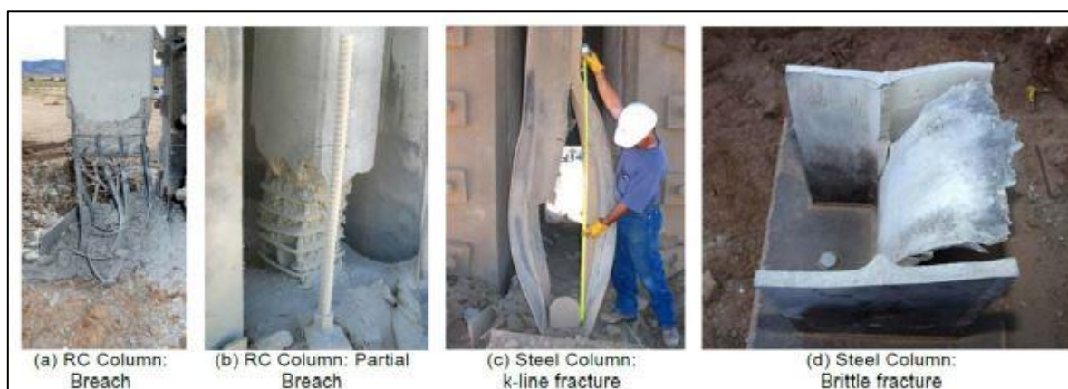
Figure 31: Column responses subject to near-contact blast charges [T. Brewer et al. 2016].
