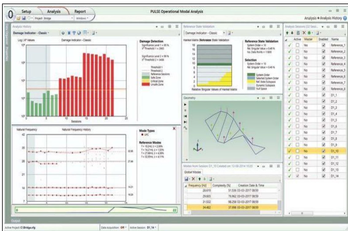
Figure 6: Damage detection of bridge by operational modal analysis [Brueel & Kjaer manual: Type 8760-8762; OMA Pro BZ: 8553].
