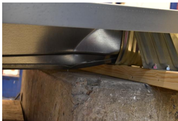
Figure 3.27. Failure of 1.50mm Test Set-up 2
