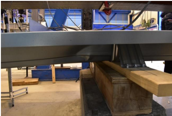
Figure 3.18. Failure of 1.00mm Test Set-up 1
