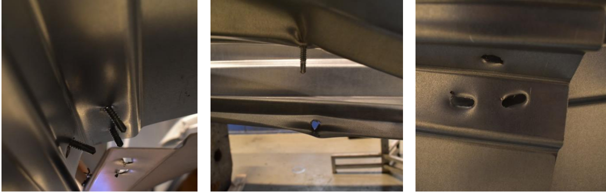
Figure 3.15. Failure of 0.85mm Test Set-up 2
