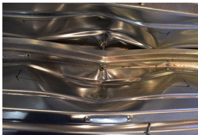
Figure 4.30. Width of web buckling for 1.50mm sheet, Test Set-up 2
