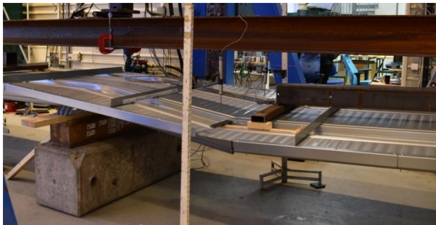
Figure 3.32. Global mechanism for Test Set-up 2, 1.00mm thick sheet
