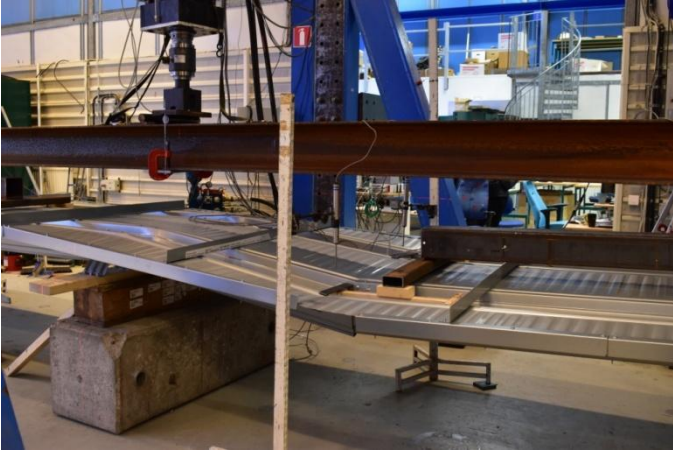
Figure 3.21. Failure of 1.00mm Test Set-up 2
