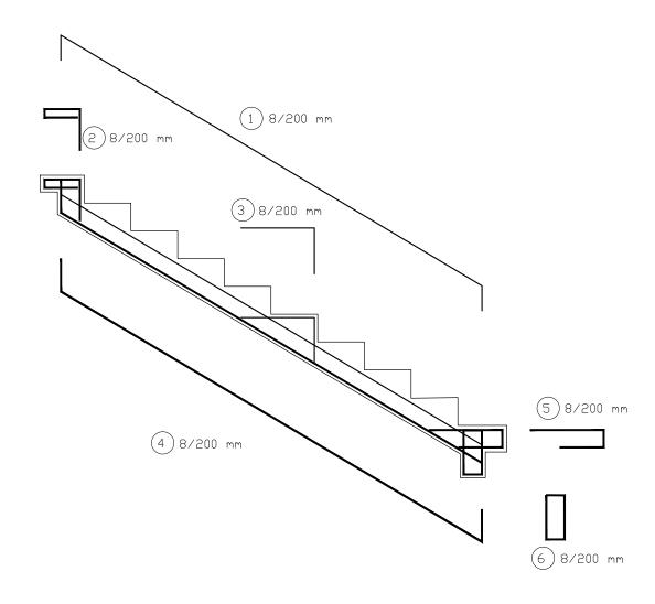
CONCRETE: C30/37-XC1-S4, Dmax = 22 mm, cl < 0,2%
