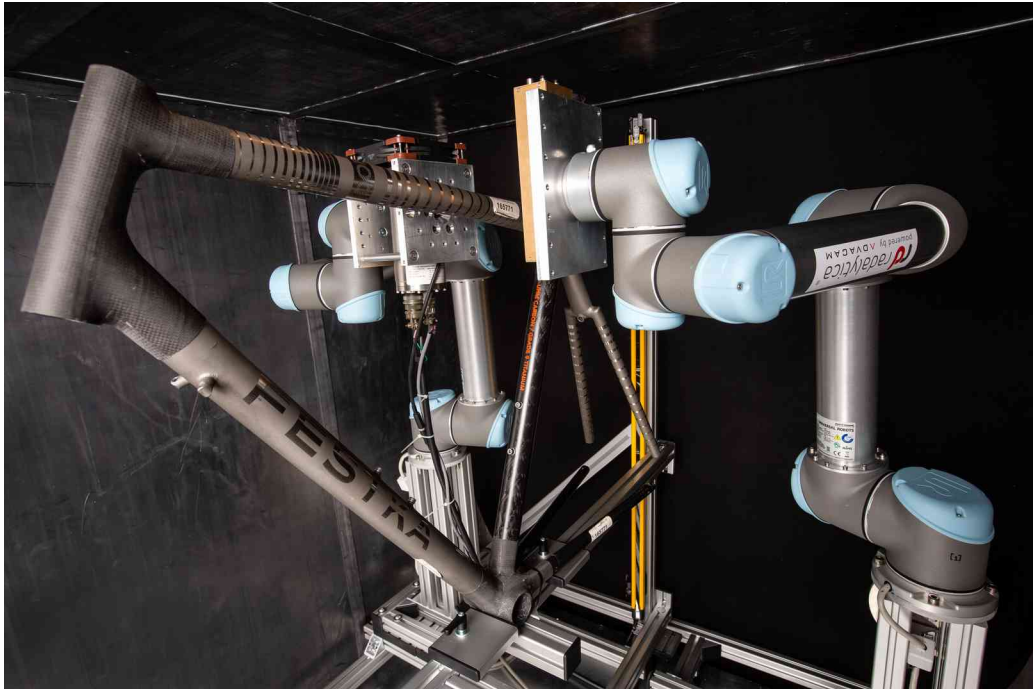
Figure 1: Dynamic system with sinusoidal nonlinearity and varying payload. The robots switch between different tools. Also, the robot on the left carries x-ray tube with a high voltage cable which changes the payload significantly during the motion. X-Ray Imaging Robotic System (credit Radalytica s.r.o.) 1
