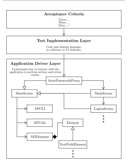
Figure 3.2: The domain model of the Application Driver Layer
