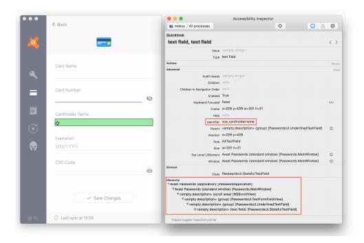
Figure 2.4: Usage of the *Accessibility Inspector* tool to determine the accessibility identifiers of the UI elements
