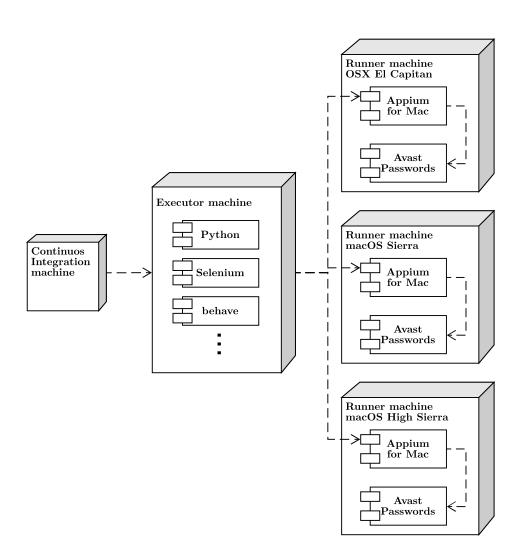
Figure 3.6: The integration of the test suite into the *Continuous Integration* pipeline
