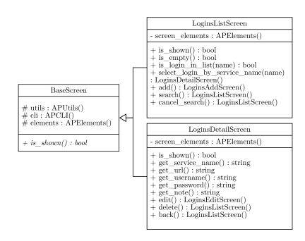
Figure 3.4: Class diagram of the *login list screen* and *login detail screen* (*page objects*) of the application
