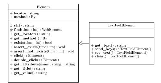
Figure 3.3: Class diagram of the Element class and one of its subclasses-TextFieldElement
