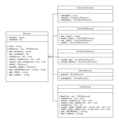
Figure C.1: Class diagram of Element class and all of its subclasses
