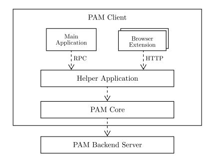
Figure 2.2: The different components of *Avast Passwords for Mac* as well as the main interactions that occur between them
