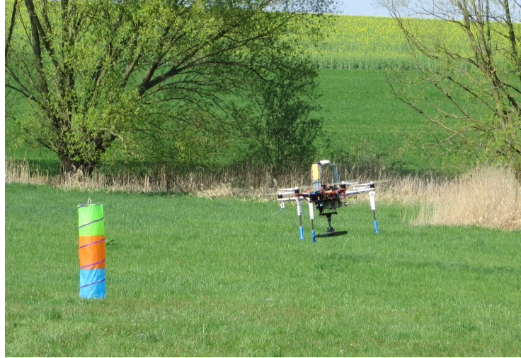
Figure 25: An MRS team’s DJI FlameWheel550 UAV equipped with a magnetic gripper carrying a metallic disc as payload, flying close to a colorful pole which marks the target.
