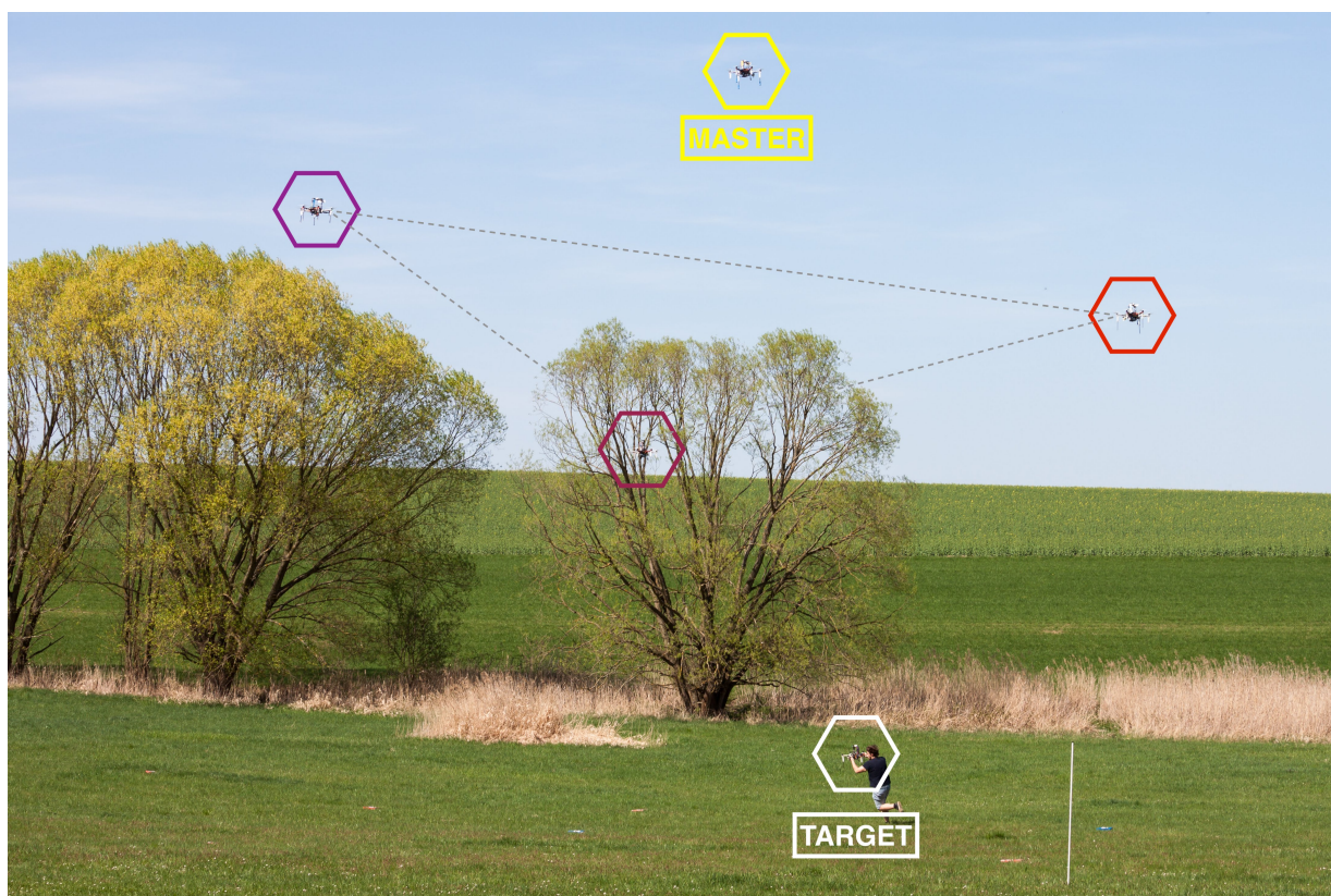
Figure 15: Photo from the real-world experiment. The target UAV was carried in hands, creating xy trajectories measured by the RTK module. The formation is tracking the estimated location from RTK to test the precision and time delay of the localization.
