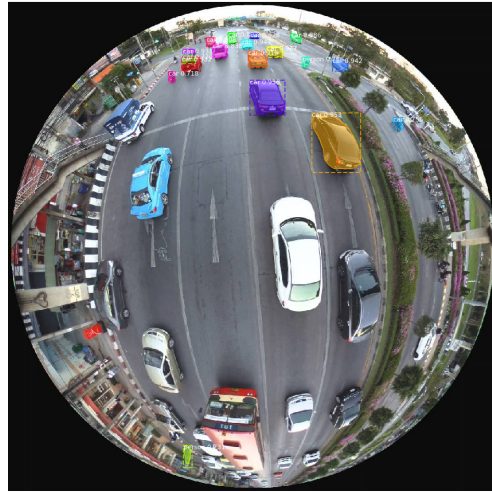
(b) Mask R-CNN on a fisheye camera has problems recognizing vehicles from the top.
