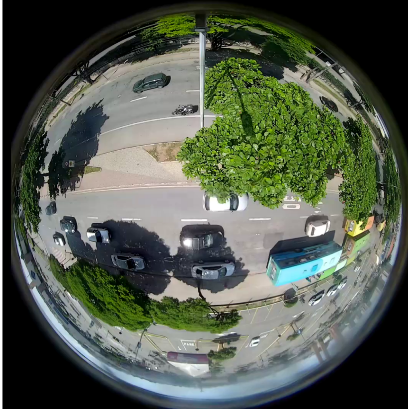
Figure 1.1: The fisheye camera is mounted in a lamp, therefore the view is directly from above.
