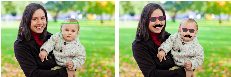
Figure 4.19: Detected faces using Viola-Jones algorithm with predicted facial keypoints on the left and altered image on the right.
