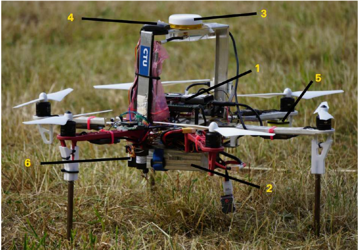
Figure 2: MAV used in real platform experiments equipped with an essential list of components. (1) computer running ROS, (2) battery, (3) differential GPS, (4) standard GPS (for the case of differential GPS malfunction), (5) rangefinder (6) Garmin rangefinder (for the case of ranger rangefinder malfunction) [18].
