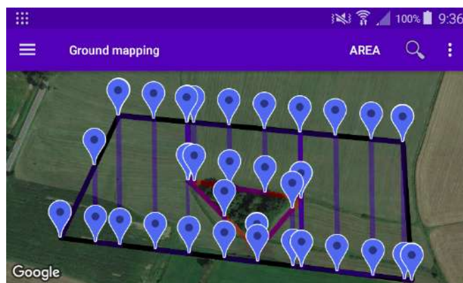
Figure 18: Generated trapezoidal trajectory represented by blue markers.
