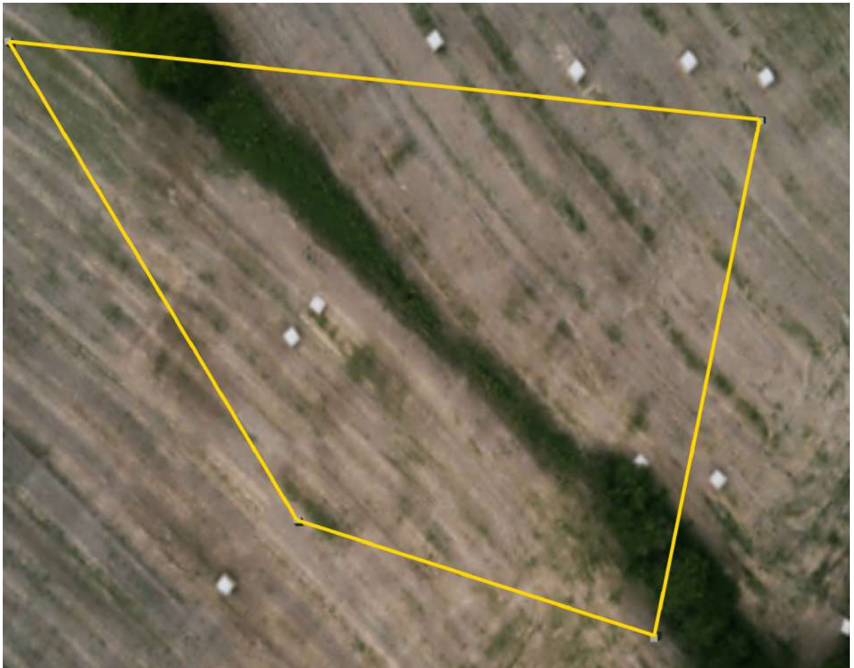
Figure 74: Result of the OpenCV stitching algorithm applied on photos taken during mapping using the Zigzag algorithm.
