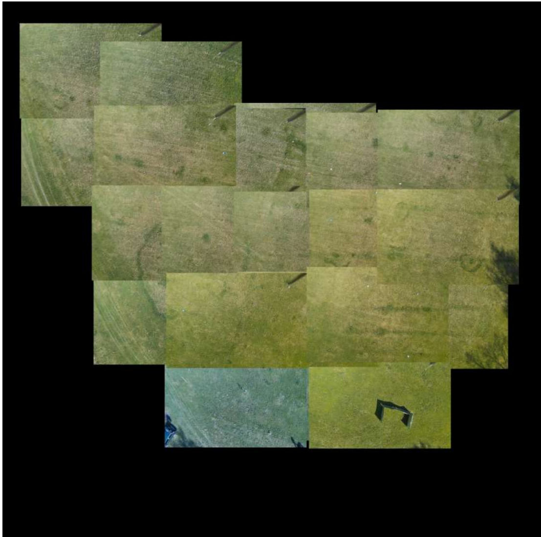
Figure 81: Demonstration of the Wavefront algorithm in a real system, while mapping an area from the altitude of 15m.
