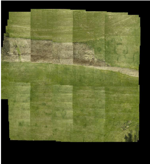
Figure 61: Demonstration of the Trapezoidal algorithm in a real system, during mapping an area from an altitude of 10m. Full image - Figure 79.
