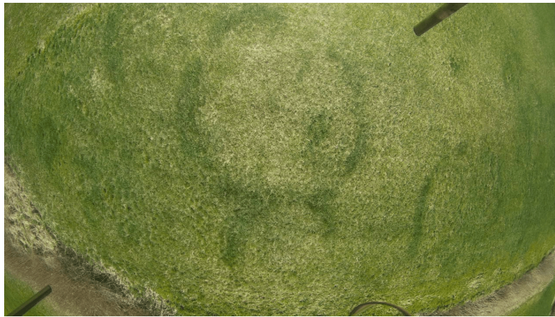
Figure 23: Example of a camera image without a rectification process. Notice the fisheye effect on the edges of the photo.
