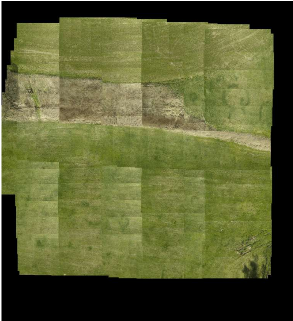
Figure 79: Demonstration of the Trapezoidal algorithm in a real system, during mapping an area from an altitude of 10m.
