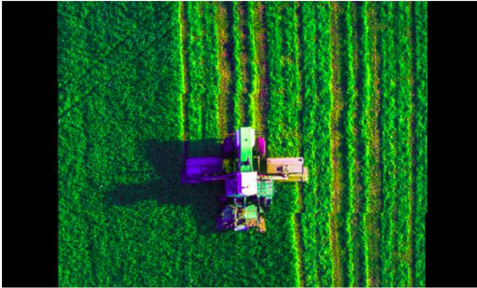
Figure 40: Result of the ZigZag mapping algorithm in the Gazebo simulation stitched using the presented sensor based stitching approach.
