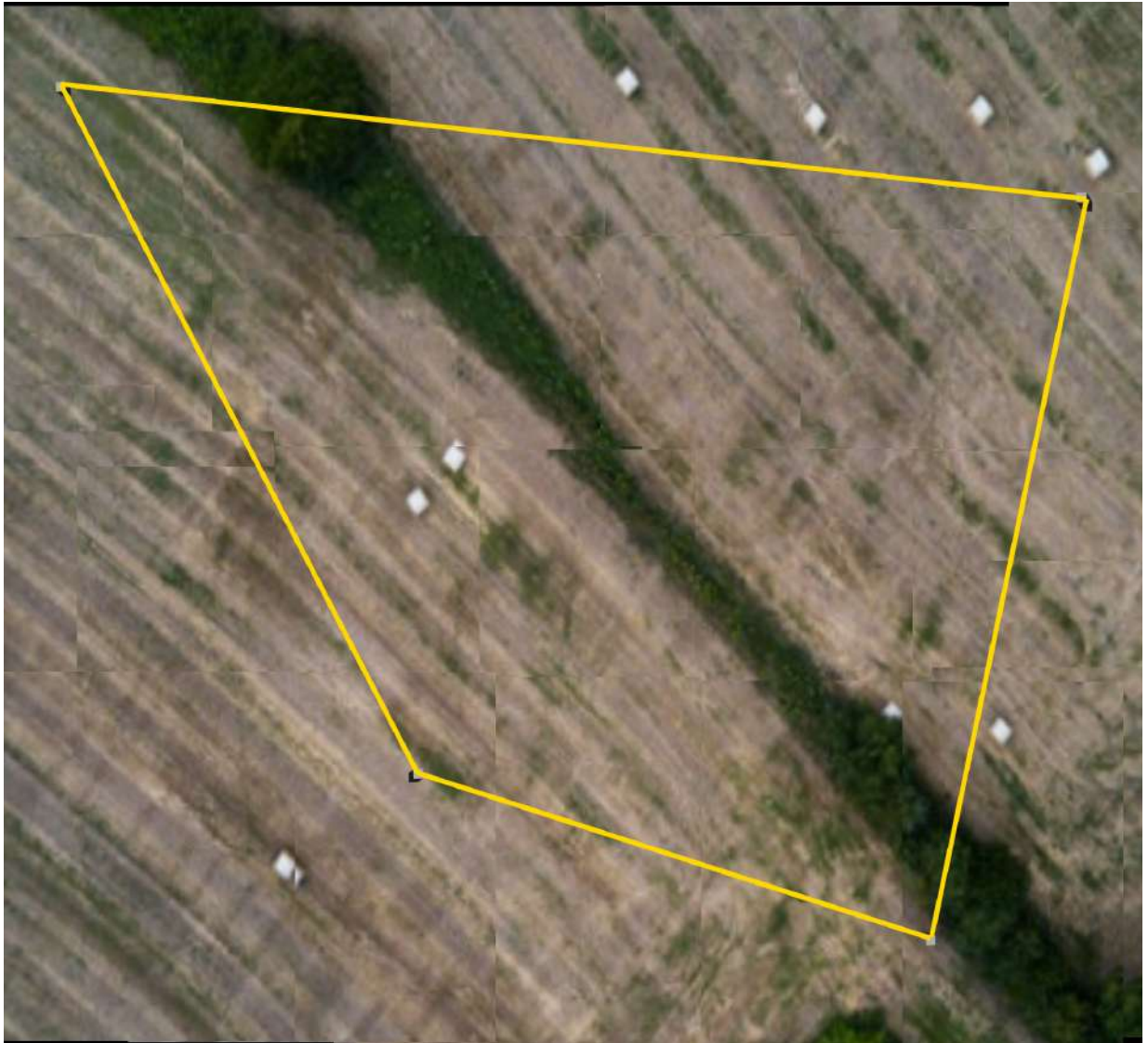
Figure 72: Result of the sensor based stitching of mapping by Zigzag algorithm
