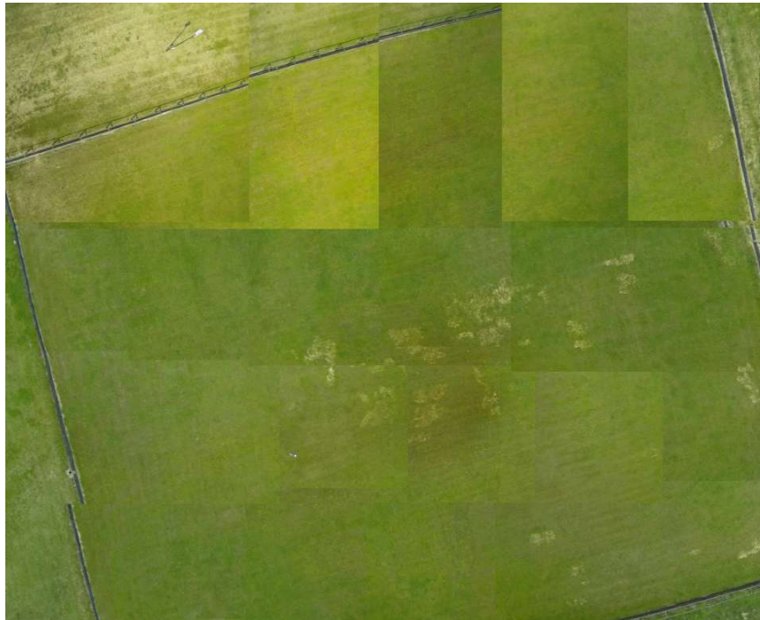
Figure 66: Demonstration of the ZigZag algorithm in a real system, while mapping an area from the altitude of 20m. Full image - Figure 84.
