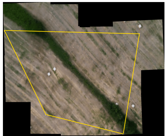
Figure 45: Result of the OpenCV stitching algorithm applied on photos taken during mapping using the Wavefront algorithm. Full image - Figure 71.
