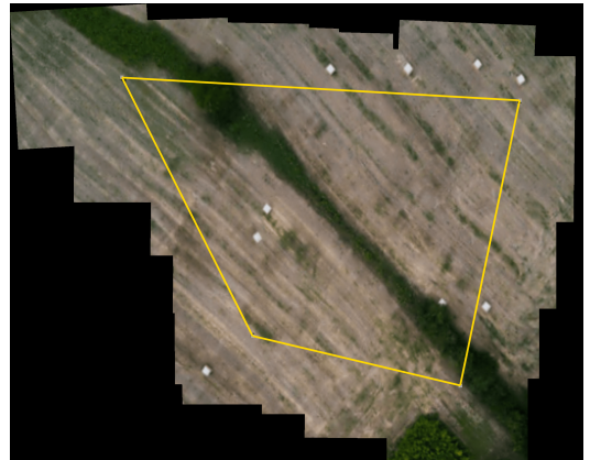
Figure 53: Result of the OpenCV stitching algorithm applied on photos taken during mapping using the Trapezoidal algorithm. Full image - Figure 77.
