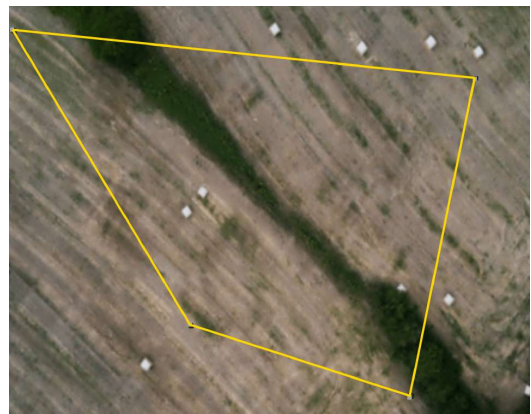
Figure 49: Result of the OpenCV stitching algorithm applied on photos taken during mapping using the Zigzag algorithm. Full image - Figure 74.
