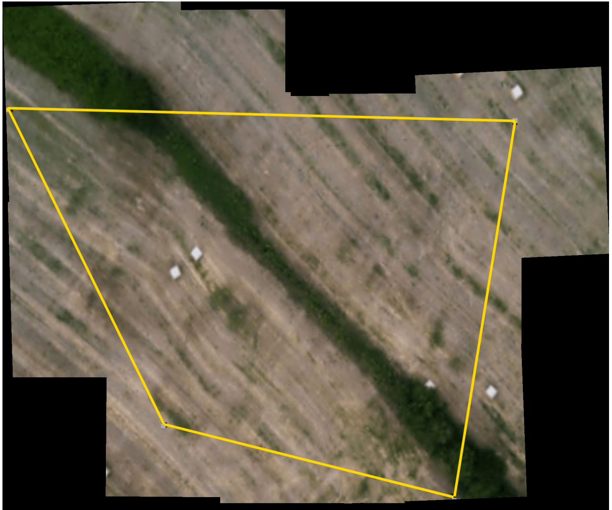
Figure 71: Result of the OpenCV stitching algorithm applied on photos taken during mapping using the Wavefront algorithm.
