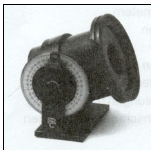
Fig. 7: Tube-adapter for external photometer head with iris-baffle and angle scale for field limitation
