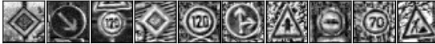
Figure 4.3: Example of the same images as in Figure 4.2 after application of all preprocessing steps — leaving out the colour information, transformation to floats in range [0, 1] for higher precision and equalization of the histogram (the transformation to floats is not important here just yet). Most notably, the advantage of histogram equalization should be obvious on first sight.
