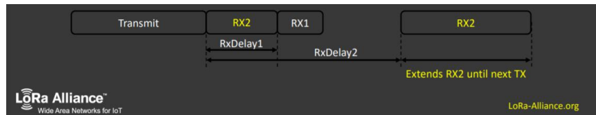
Figure 2.8: Scheme of class C communication [8]
