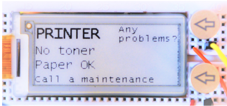
Figure 5.2: Designed system of two buttons and e-ink display
