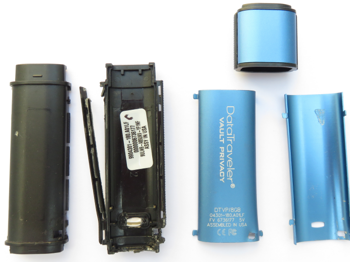
Figure 3.2: Enclosure taken apart
