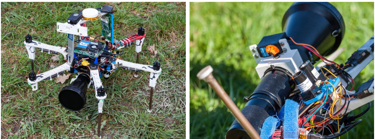
Figure 42: Interceptor equipped with a net launcher (left), and net launcher servo triggering mechanism (right).
