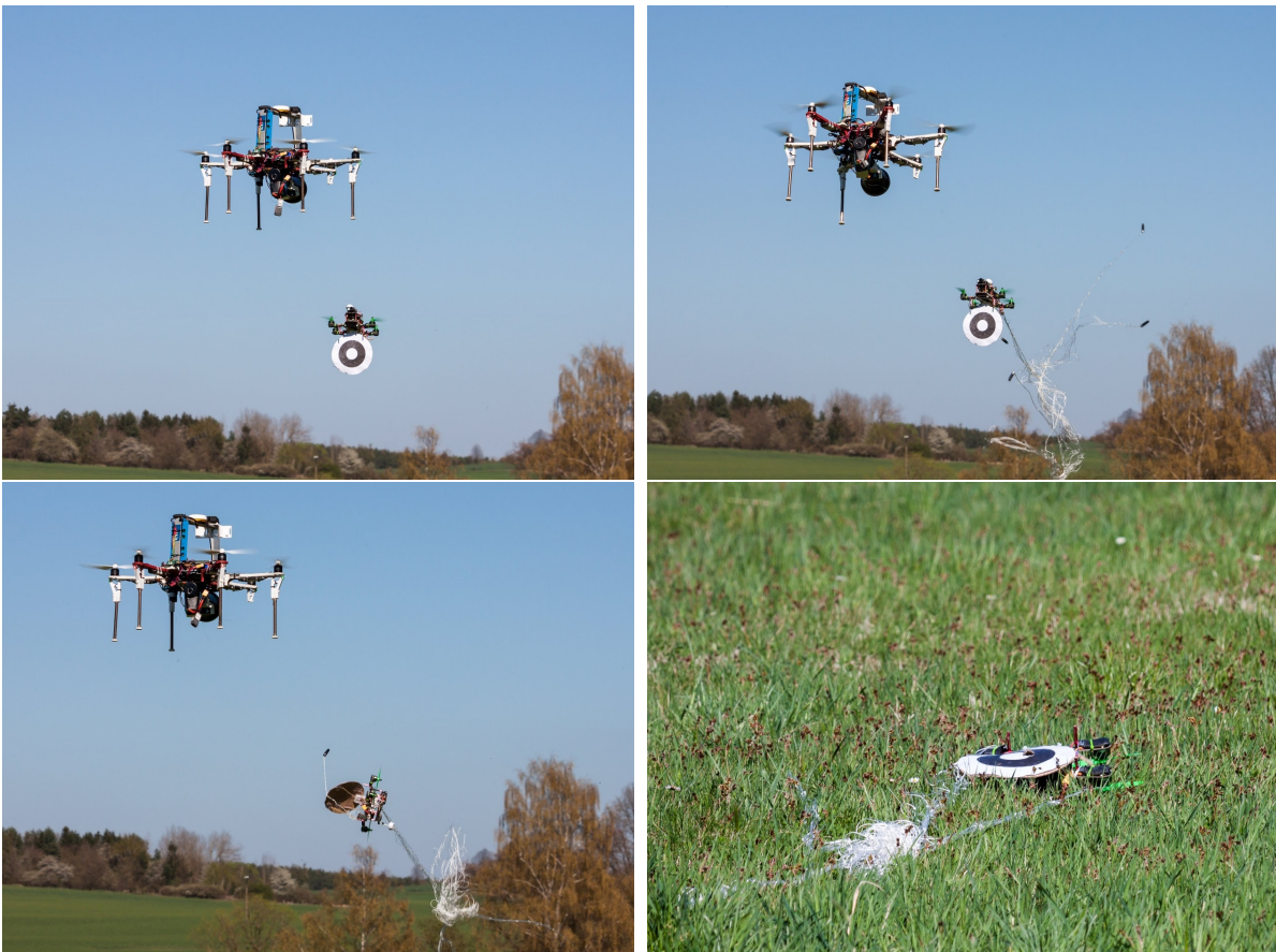
Figure 45: The interceptor launching a net and hitting the target.
