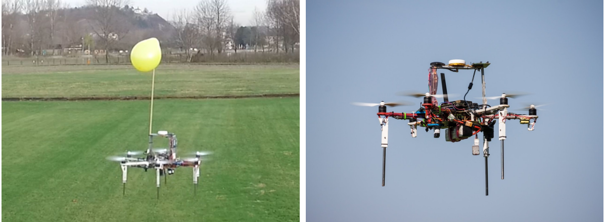
Figure 35: The target drone fitted with a balloon (left) and the interceptor (right).
