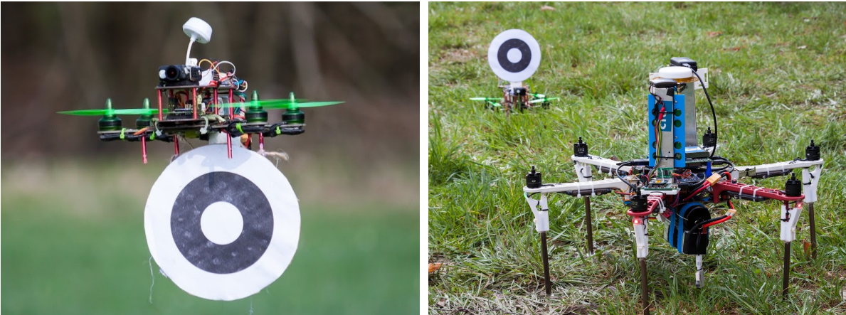
Figure 43: The target in flight, equipped with the WhyCon pattern (left), and size comparison between the target and the interceptor (right).
