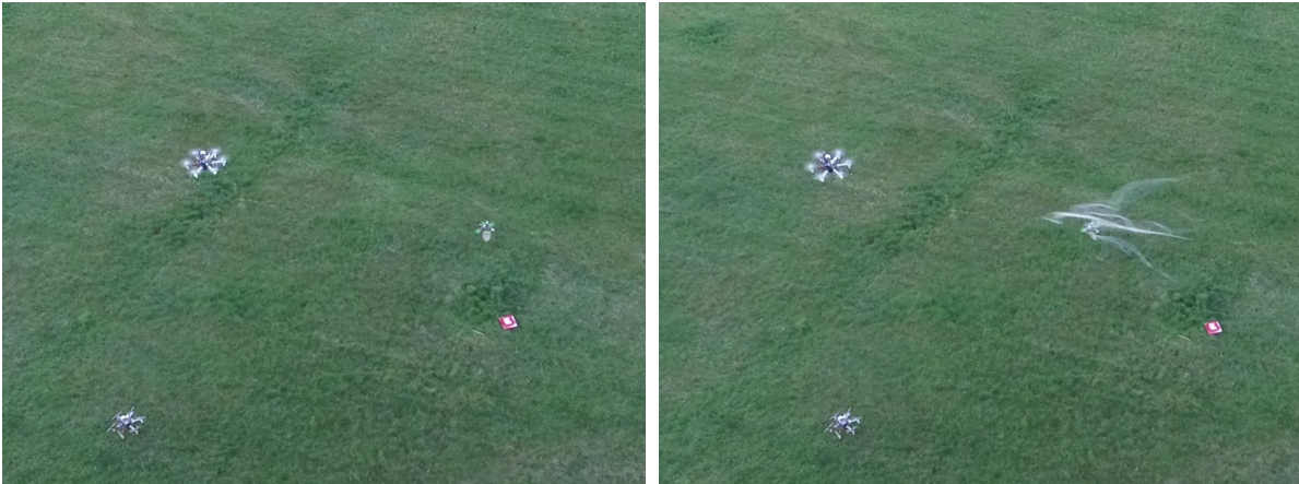
Figure 44: Target being captured by the launched net, aerial perspective.
