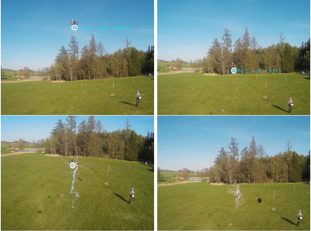
Figure 51: Dynamic target scenario from the point of view of the interceptor, including the output of WhyCon. Images have been cropped for better visibility.
