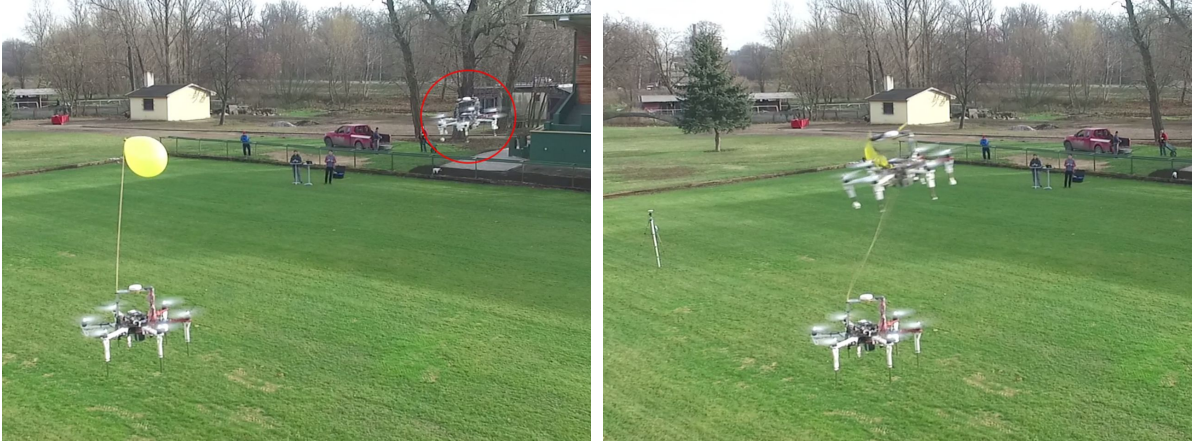
Figure 36: The interceptor approaching the target with the balloon (left) and the interceptor popping the balloon (right).
