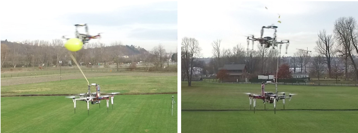
Figure 37: Interceptor attacking the balloon mounted to a static target.
