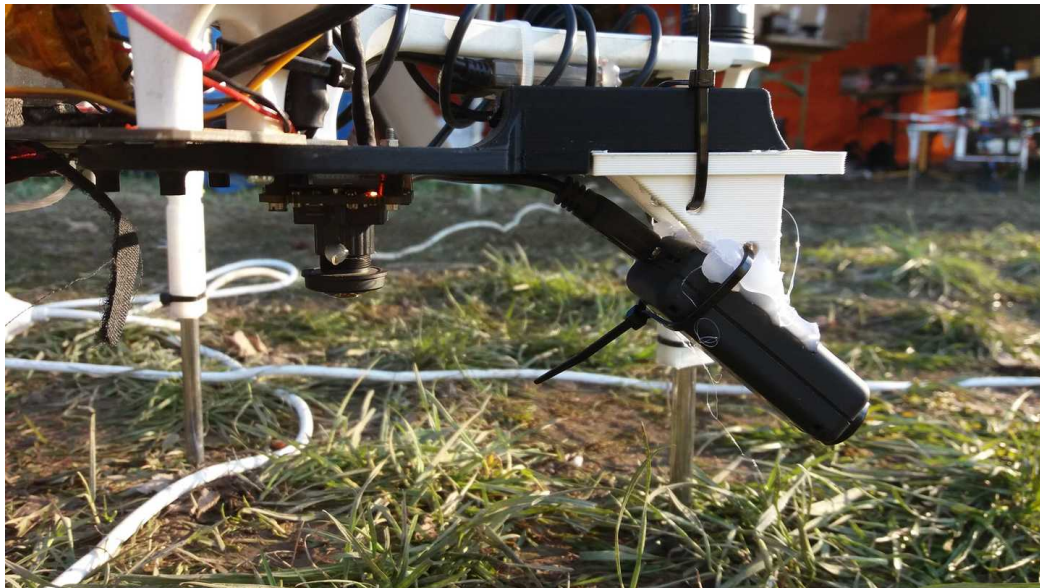
Figure 30: The Mobius camera and its holder from profile
