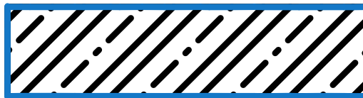
Figure 5.1: Application of Alpha shape on a diagonal line hatch inside a wall - original CAD drawing is shown in black, remaining part of the drawing after application of Alpha shape is shown in blue
