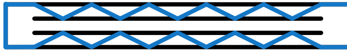
Figure 5.3: Application of Alpha shape on parallel lines inside a wall (undersampled) - original CAD drawing is shown in black, remaining part of the drawing after application of Alpha shape is shown in blue
