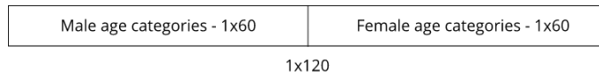
Figure 4.1: The Output of the age and gender prediction CNN. The 120-dimensional vector constitutes of two gender categories, each consists of 60 dimensions representing ages from 16 to 75. Each dimension can be interpreted as a probability of given category.
