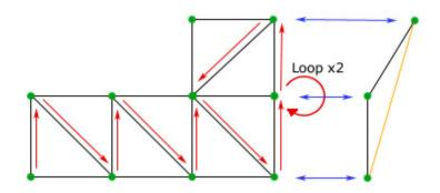
Figure 3.2. GLTriangleStrip trick allowing for drawing planes within a single strip.
