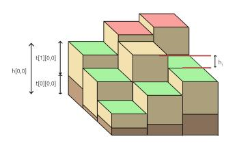
Figure 2.2. Thermal erosion - green cells will receive material, red will not.
