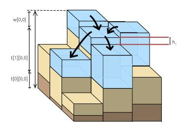
Figure 2.3. Four neighboring cells accelerating water based on surface height.
