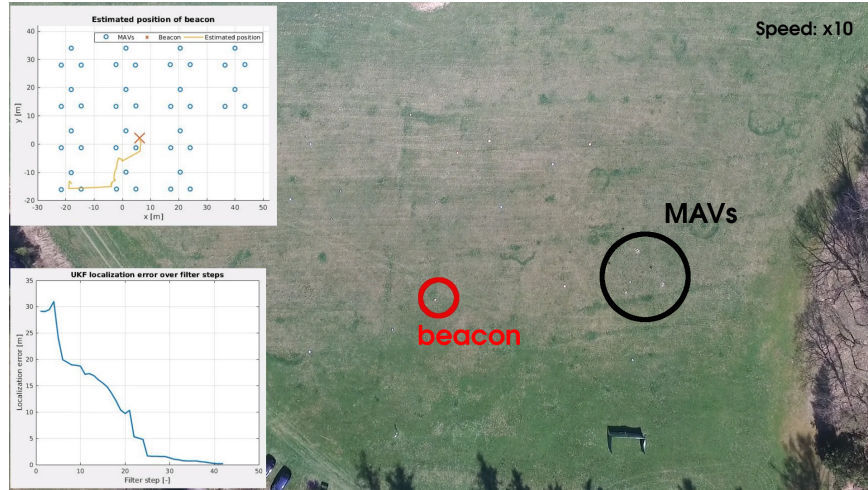
Figure 7.11: Localization of the beacon during the second flight in the experiment with MAV formation following a predefined trajectory
