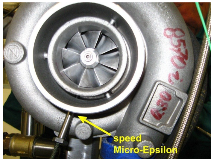
Figure 19 Detail of compressor with Micro-Epsilon sensor for measurement of turbocharger speed
