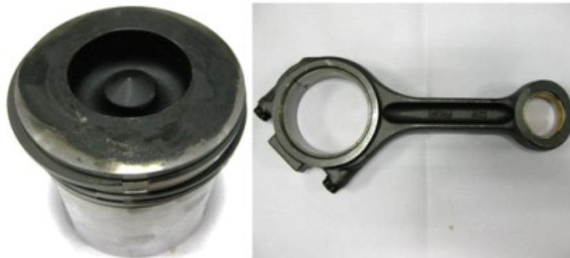
Figure 53 Piston and connecting rod of the experimental engine, example of geometrical data used in the simulation
