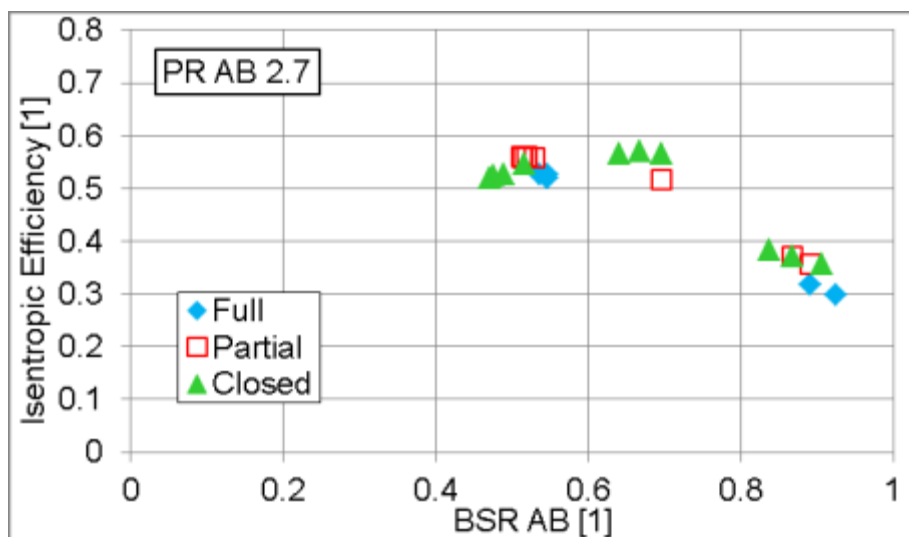
Figure 198 Comparison of turbine isentropic efficiency courses - overall pressure ratio PR AB = 2.7; full admission - blue; partial admission level A approx. 0.87 - red squares; closed section - green triangles
