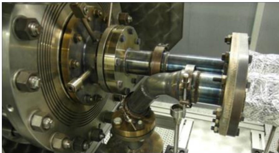
Figure 5 Double burner concept for twin entry measurement [25]
