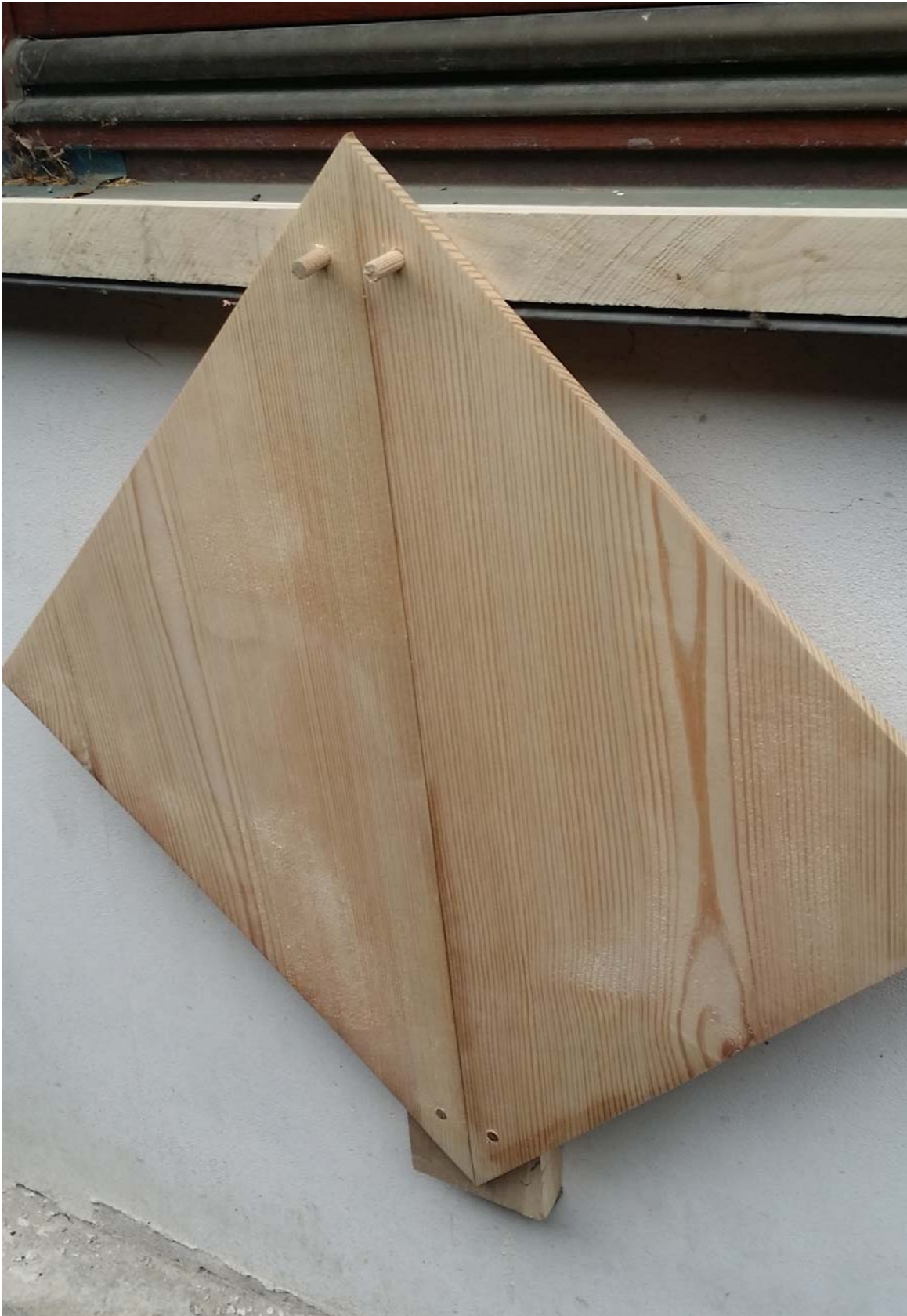
Figure 21: Test of Plugs Based on Wood's Hygroscopicity instead of Glue in Natural Environmental Conditions (photo: Bouma 2015)
