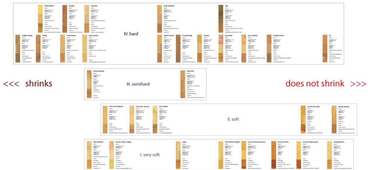
Figure 59: Davidová 2012: Map of Shrinking and Warping of Different Local Wood Species (data and most of the images from: Němec, 2005 used with the courtesy of Grada)
