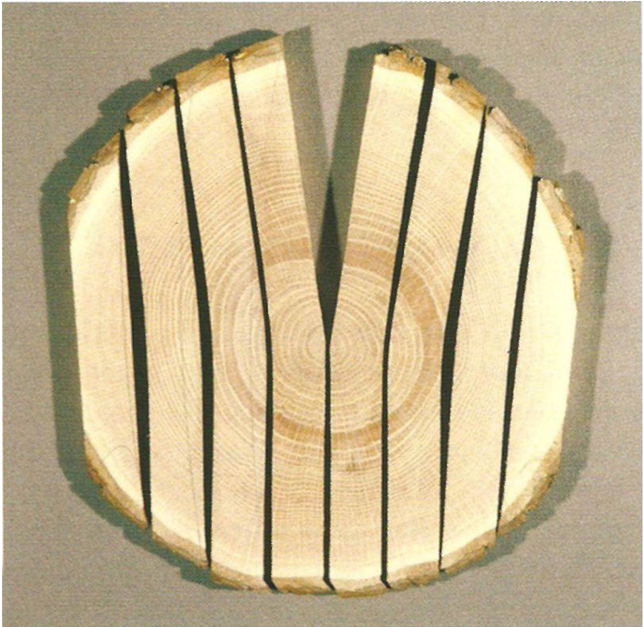
Figure 60: The Severity of Cupping in a Board is Related to its Position in the Log (photo: R. Bruce Hoadley from: Hoadley, 1980; with the courtesy of Taunton press)
