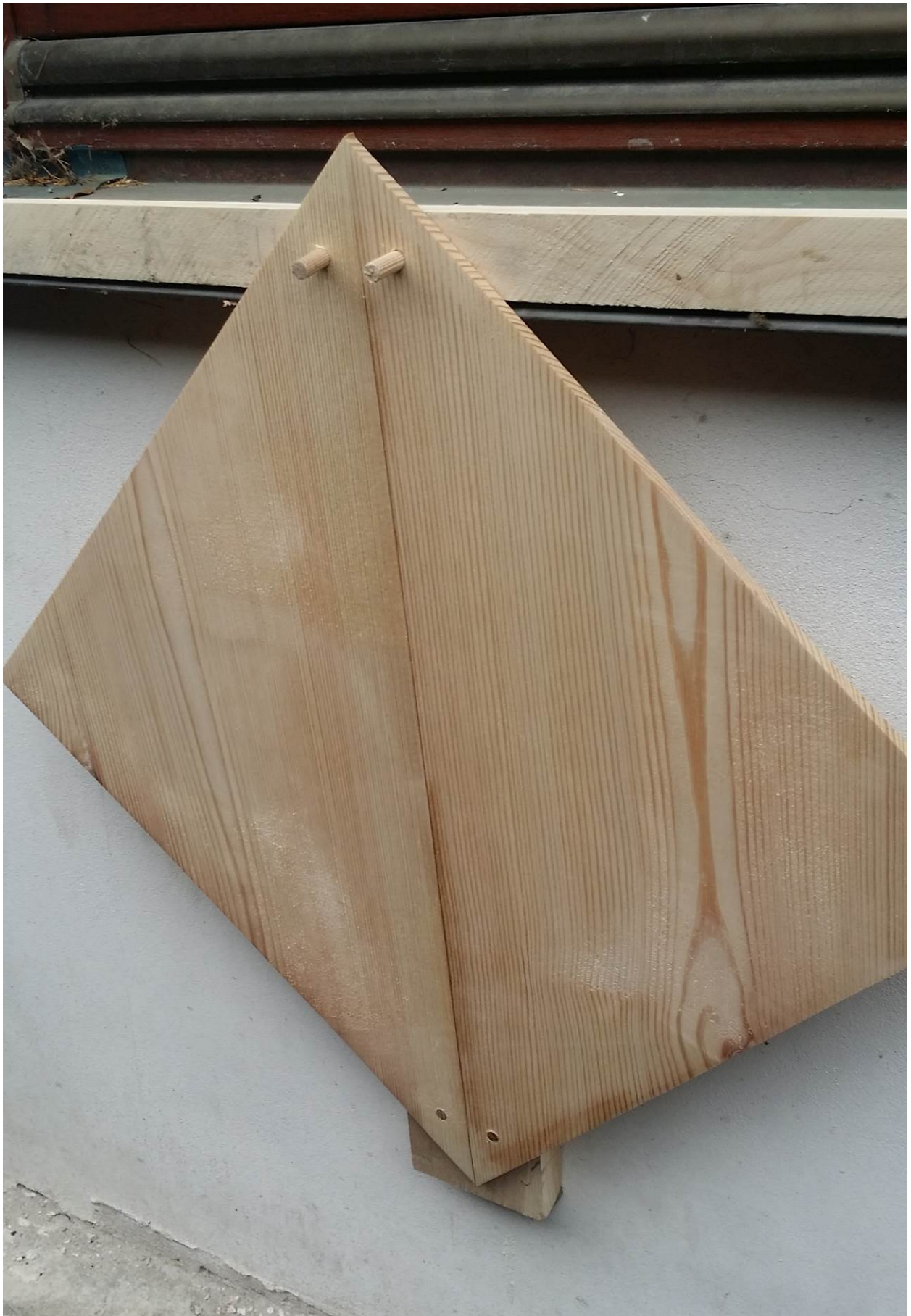
Figure 96: Test of Plugs in Natural Environmental Conditions (photo: Bouma 2015)
