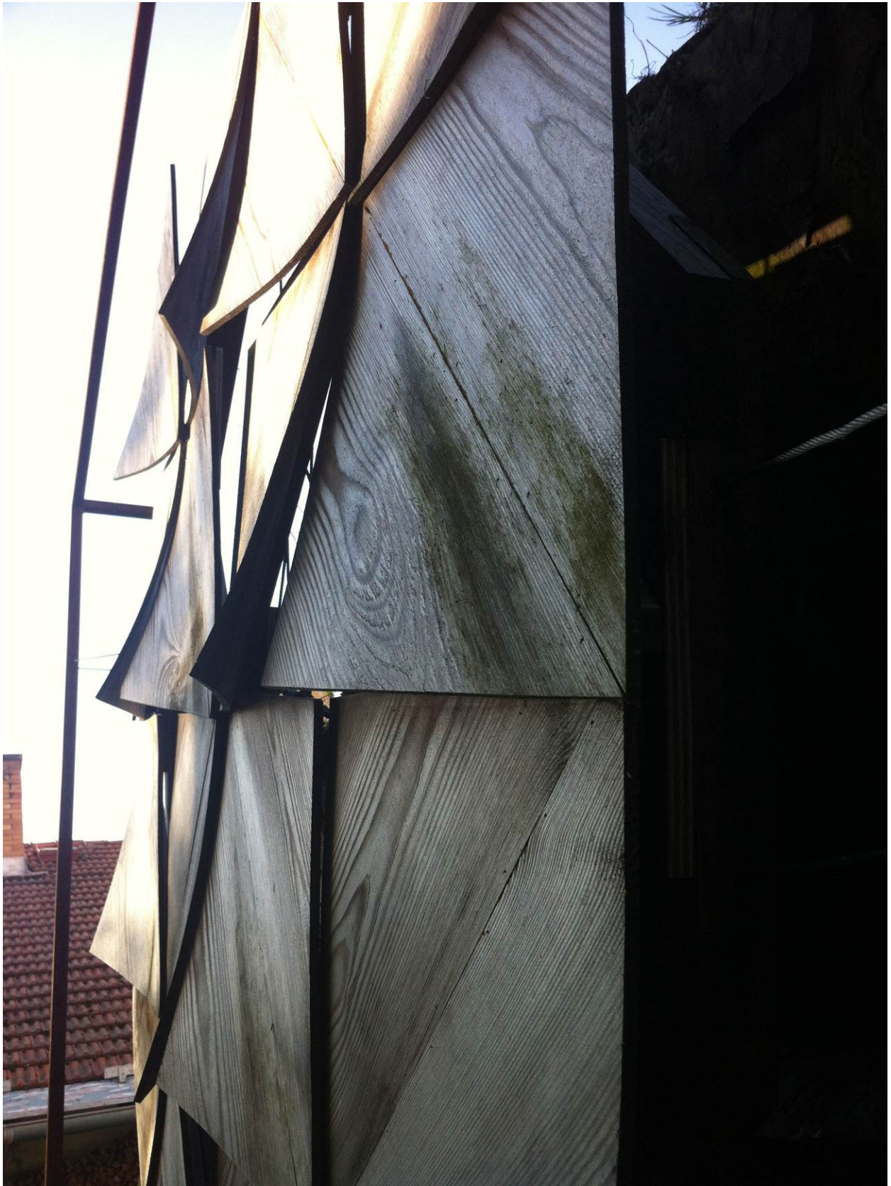
Figure 12: Ray 2 Prototype after Three Years of Being Exposed to Weather and Biotic Conditions (photo: Yildirim 2016)
