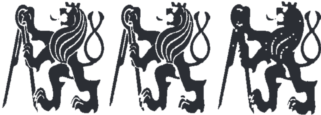
Figure 2.16: Image opening and closing. Left is the original image, in the middle, opening was performed, which led to loss of small features in the image (visible on the feet of the lion). Right is image closing. It leads to filling of the blank spaces in the image. Picture from http://cmp.felk.cvut.cz/~hlavac/TeachPresCz/11DigZprObr/71-3MatMorpholBinCz.pdf
