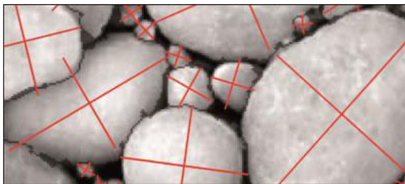
Figure 2.17: Image with depicted object axes calculated by MATLAB from the interpolation with ellipses of the same normalized second central moments as the regions of interest. Picture from https://www.researchgate.net/profile/Martin_Detert/publication/283879329/figure/fig3/AS:391565685084162@1470367942252/Figure-5-Final-result-of-object-detection-procedure-Straight-lines-colorprint-red.jpg .
