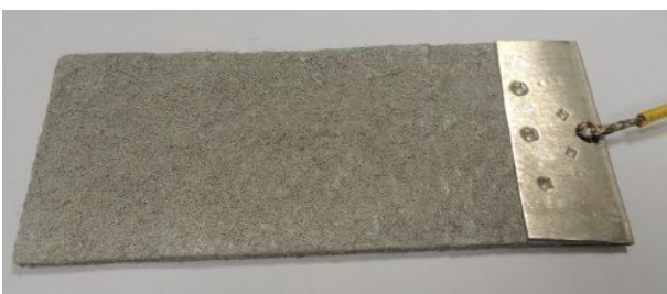
Fig. 2. Monometallic tin felt electrode ready for filling (non-woven PP textile carrier prepared by needling).
