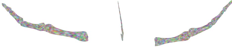
Figure 2.1: Mesh deformation caused by linear interpolation on rotating object
