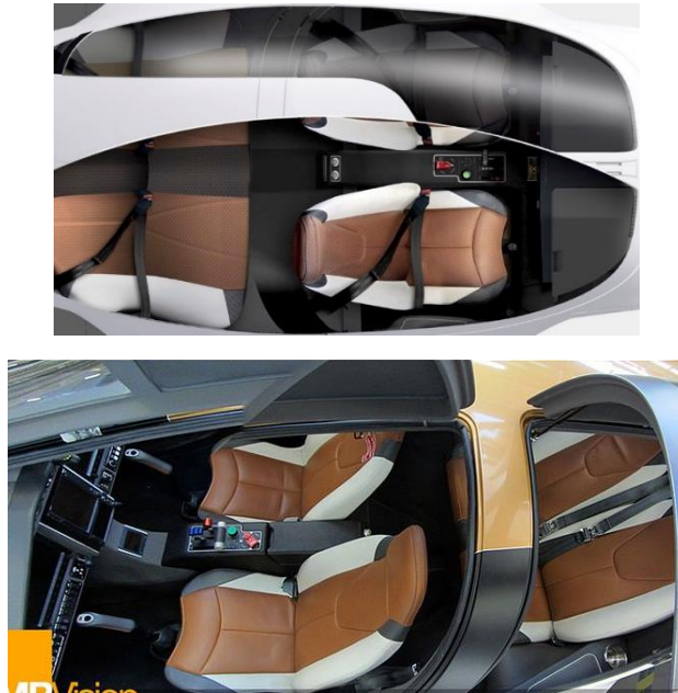
Figure 7.5. A typical 2+2 seating configuration cockpit layout. Image is showing a cabin of Pipistrel Pathera aircraft.
