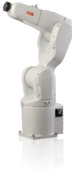
Obr. 42 robot IRB 1200 s dosahem 900 mm [30]
