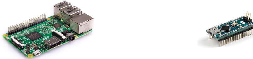
Figure 1: Raspberry Pi 3B on the left and Arduino Nano on the right
