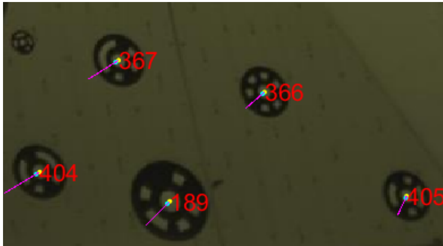
Figure 6.1 Zoom to details of reprojection errors in 2 nd slave Trifocal camera, 3 rd frame. Yellow dots are the observations u , Cyan dots are the calibration's reprojections. Magenta ray is the error vector scaled by 10x.
