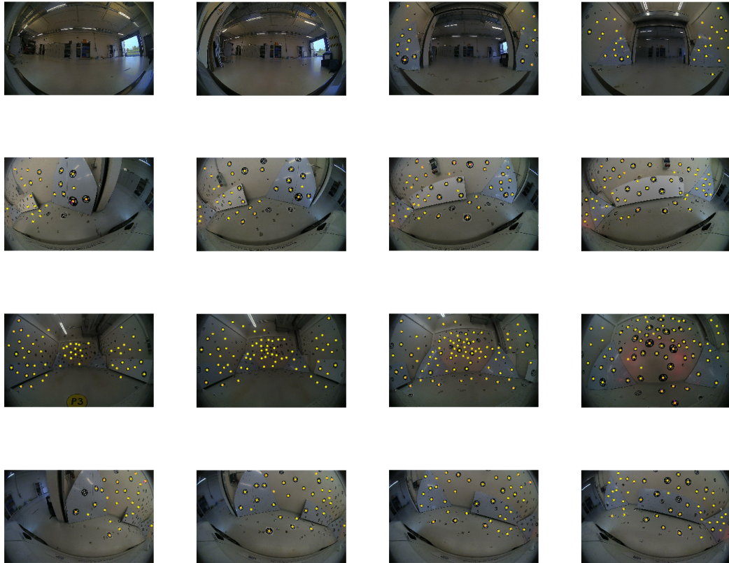
Figure 6.4 Session 2: first four cameras (see Table 6.1) (rows) in four different time-frames (columns). The Yellow dots marks the reprojection. Red dots denotes the observations u . The observations may not be fully seen if occluded by reprojection marker. The magenta rays are the residuals scaled 10x.
