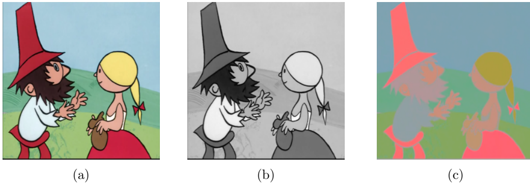
Figure 1.1: Color image (a) decomposed into (b) luminance and (c) chrominance in the Lab color space.
