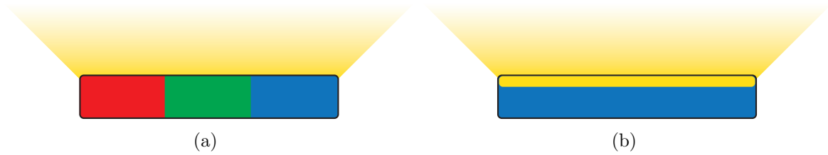
Fig. 2.3: White light generation by (a) combining three individual RGB emitters and (b) covering yellow phosphor layer over a blue LED chip. Note, that the emitted colour is indicated in yellow to improve visibility, but in reality the emitted light is white.
