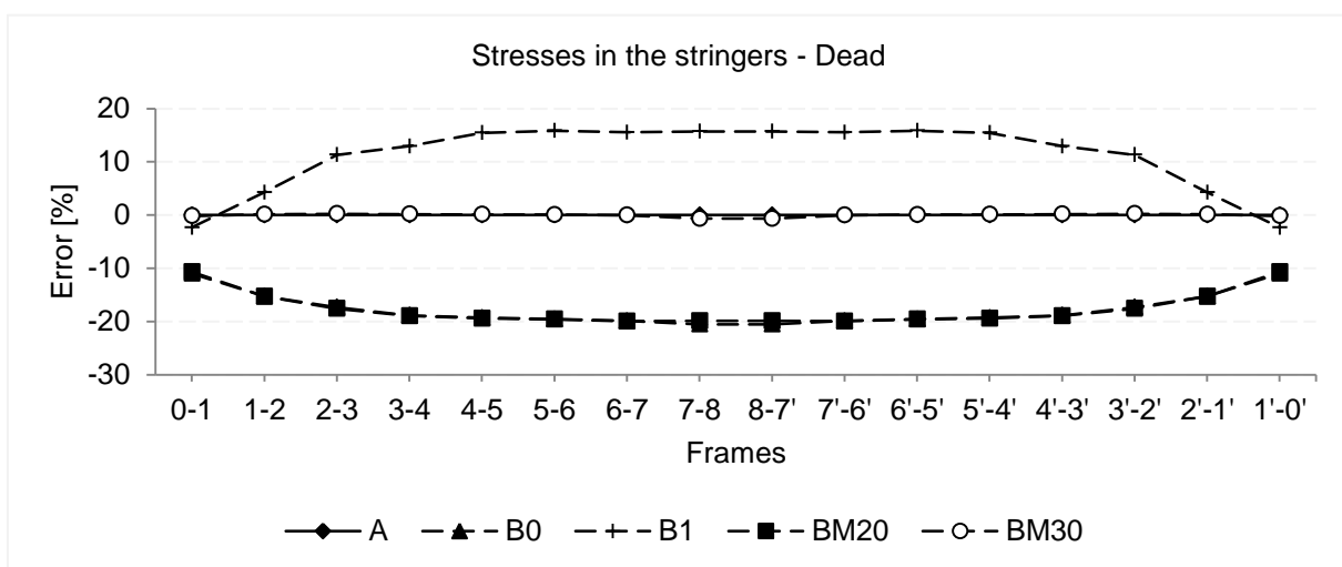
Figure 63. Stresses in stringer for different conditions on connections of crossbeams.
