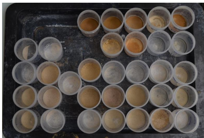
Figure 6: Example of collected and dried mass loss during wetting
