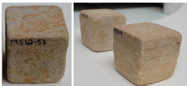
Figure 17: Mšene Test 3 (partial immersion) - heterogeneous deterioration
