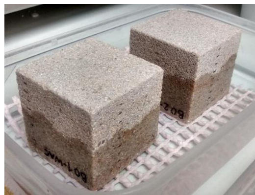
Figure 14: Aspect of Božanov stone during the capillary test revealing the heterogeneity of the stone as seen from the tortuosity of the wet front.
