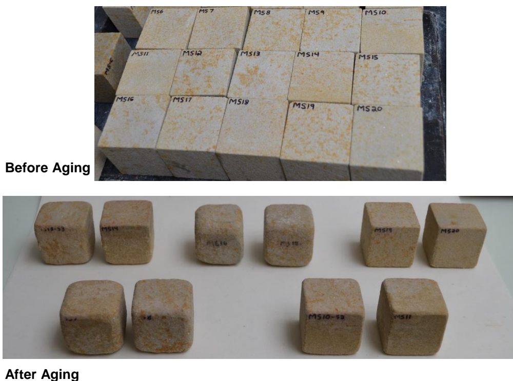
Figure 16: Comparison of Mšene before and after salt aging cycles
