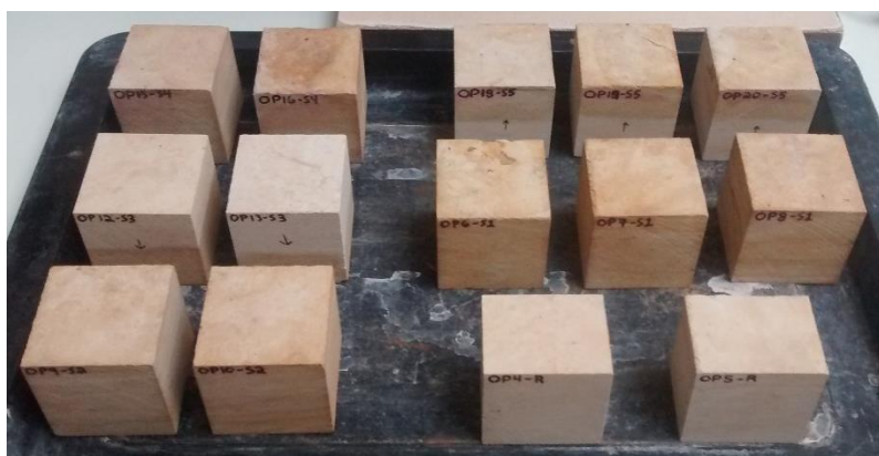
Figure 18: Colour change after one cycle with all test procedures in Opuka stone.
